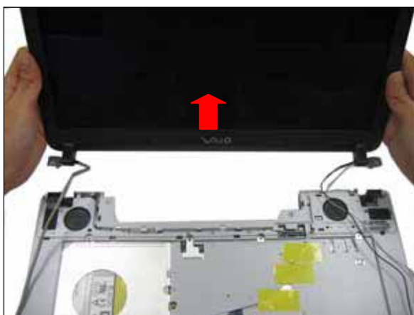
Step 18. Gently remove the LCD in the direction of arrow and set aside.
