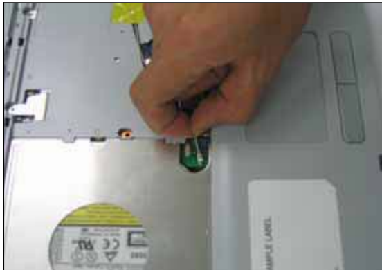
Step 15. Gently Pull out the black and white cable.
