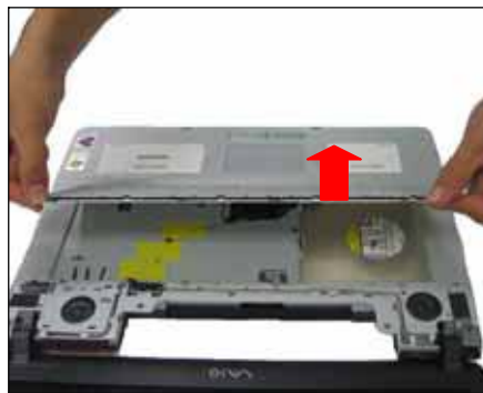
Step 12. Remove the keyboard in the direction of arrow.
