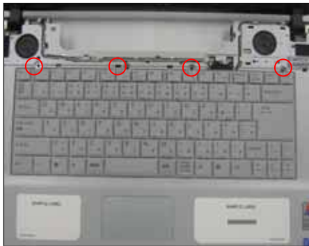
Step 11. Using a screwdriver remove the marked screw.
